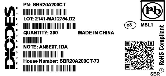
Fig. 3: Standard Label for SBR® Product that has Lead-Free Finish and is RoHS Compliant with Tin terminal finish. Moisture Sensitivity Level 1.
