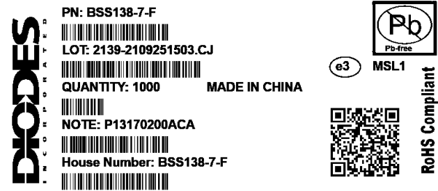
Fig. 5: Standard Label for a totally Lead-Free product, RoHS Compliant Product with Tin terminal finish and Moisture Sensitivity Level 1.
